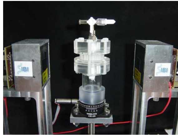
Fig. 1. Photograph of the microPET system showing the two detector modules, with a microDerenzo phantom on the rotation platform, midway between the modules.
