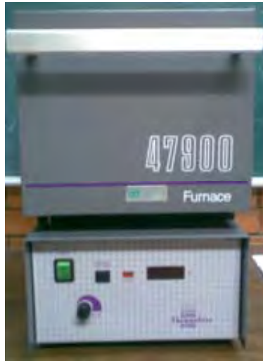
Figura 5.3. Horno Thermolyne, Furnace 47900.
