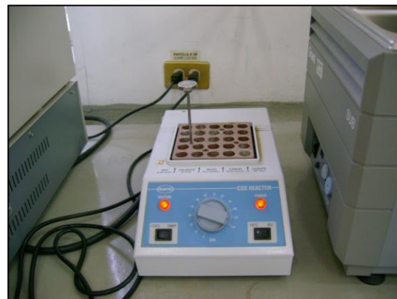
Figura A4.5.b. Digestor
