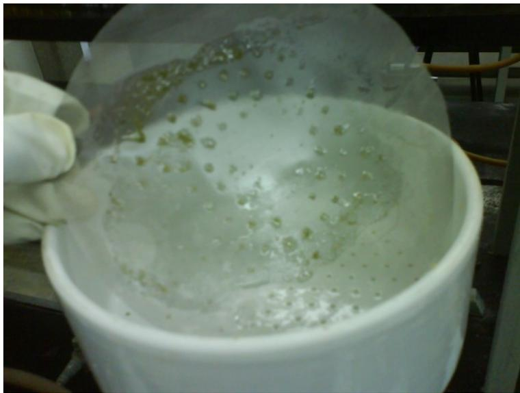
**Figura 4.4 Tamiz de 20  $\mu\text{m}$**
