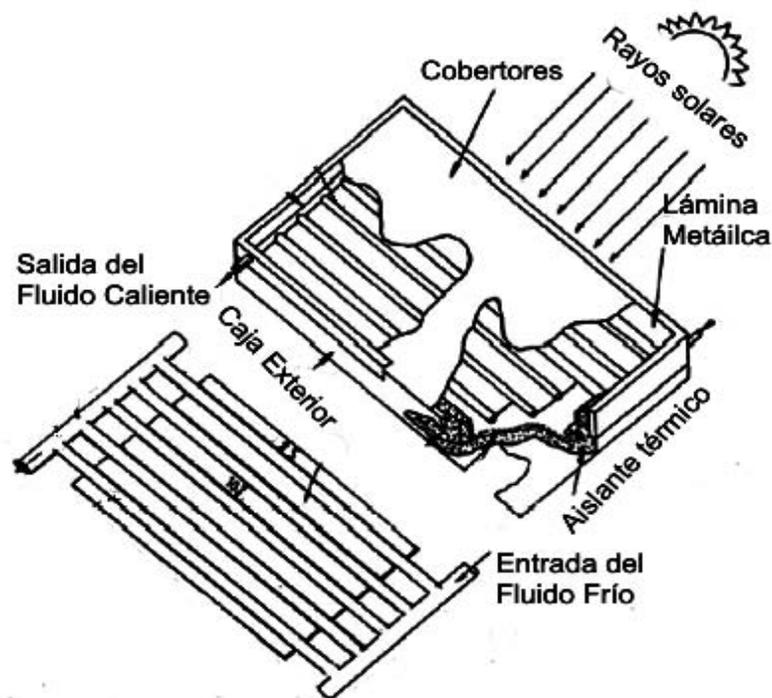
Figura 7. Colector solar plano<sup>4</sup>.
