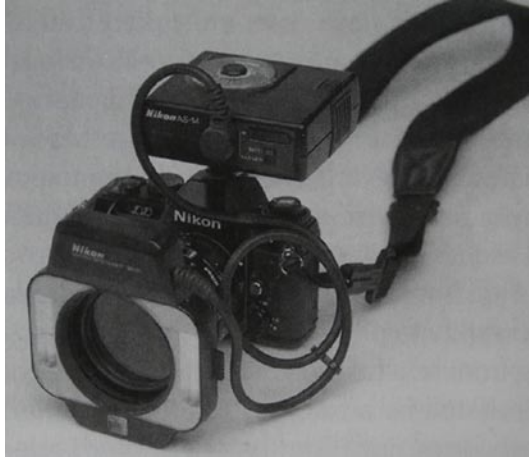
Ring Flash o Flash de arillo (Lawrence B. Stack, "HANDBOOK OF MEDICAL PHOTOGRAPHY" pág. 6)
