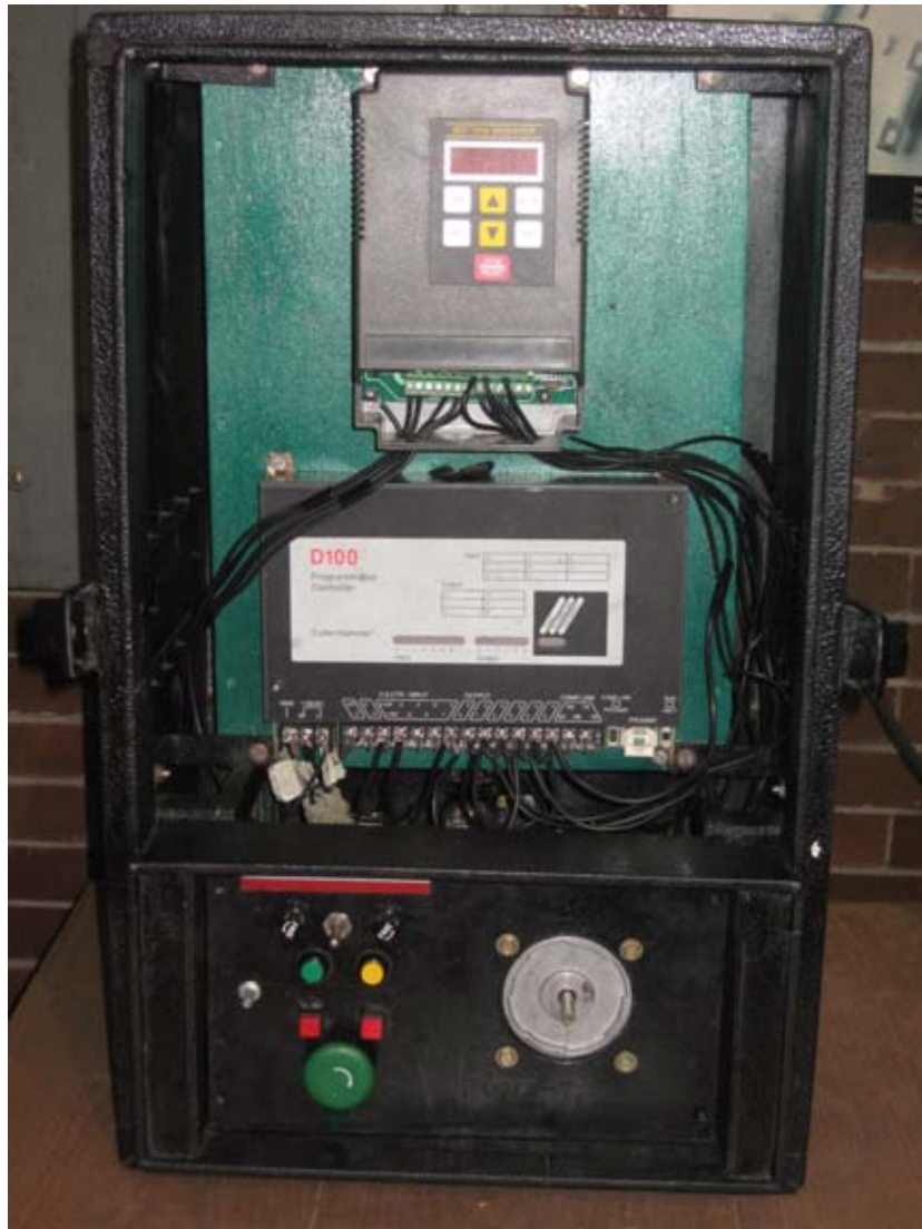
Figura 142 Sistema PLC – Drive – Motor.
