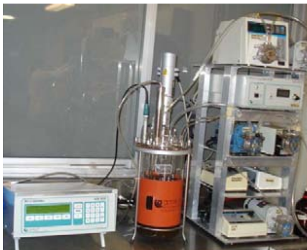
Figura 4.4 Reactor anaerobio SBR
