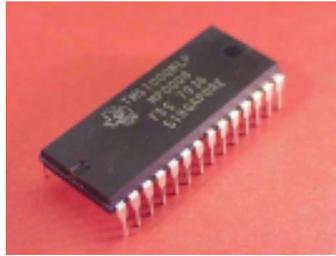
Figura 2.2. Microcontrolador Texas Instruments TMS1000.
