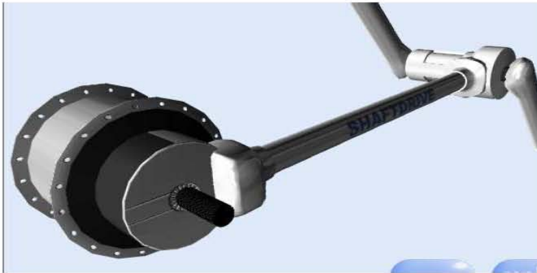
Fig. 3.3 Sistema de cardán (Shaft Drive).
