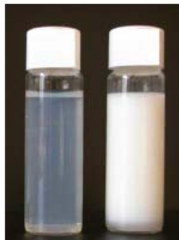
Fig. 1. Picture of a nano-emulsion (left) and a macro-emulsion (right) with droplet diameters of 35 nm and 1 \mu m, respectively.
