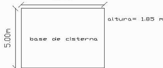
CISTERNA DE CONCRETO ARMADO, CAPAC. 46,000 Lts.
