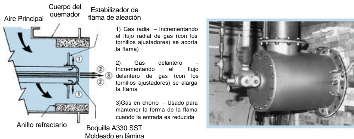
Figura 6.2 Quemador Marca North American Manufacturing Company Modelo 4384.
