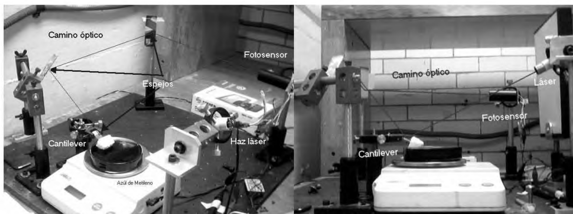
Fig.1 and 2. In these figures the experimental arrangement is presented for the detection of the variation of the height of the level on the liquid that is inside a glass recipient, by means of the deflection of the laser beam that is directly focused toward the cantilever, on the cantilever it has been placed a mirror like initial part of the optic path of three mirrors, which directs the beam towards the entrance position of the photosensor.
