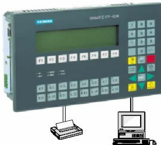
Figura 2.2 Controlador lógico programable. (GEA Liquid Processing Division) 8
