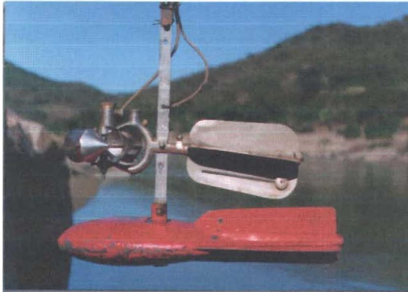
FIGURA 2.1. MOLINETE HIDRÁULICO
