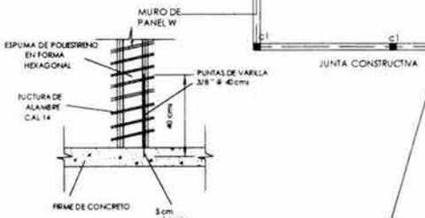
**CORTE DEL MURO ESTRUCTURAL 3"**
