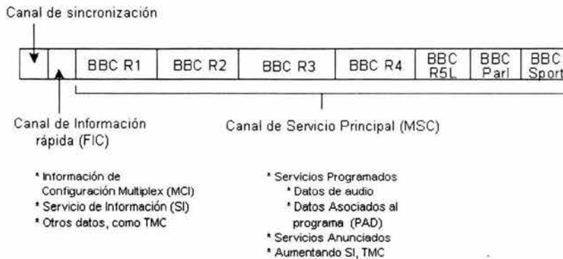
Fig.1.8 Multiplexado DAB
