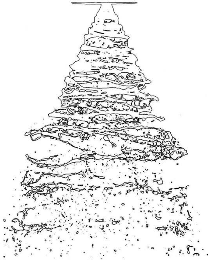
Fig. 5 Image showing the resulting contour of the spray in Fig. 3 when the filtering is done at half the maximum intensity value.
