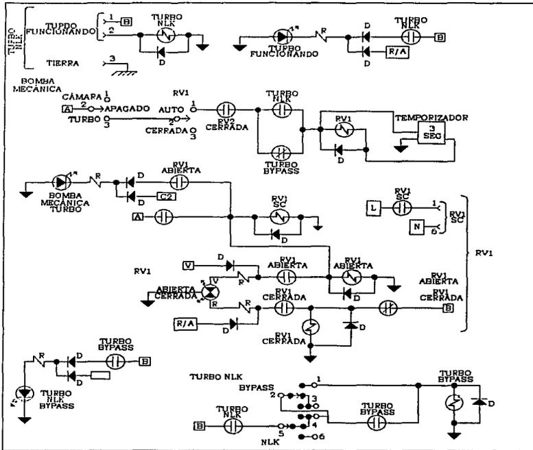
Fig. 3.5 DIAGRAMA ELÉCTRICO PARA RV1
