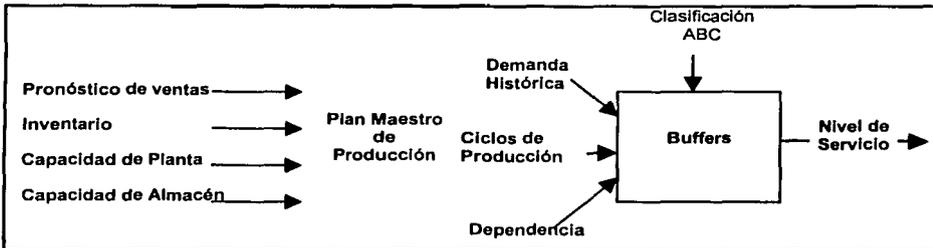
Figura 4. Esquema de Buffer Management.
