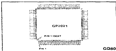
Fig 1. Pin Connections - Top View
