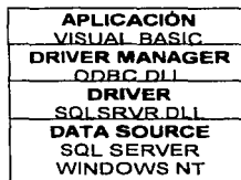
Figura 4. Arquitectura del Open Database Connectivity.
