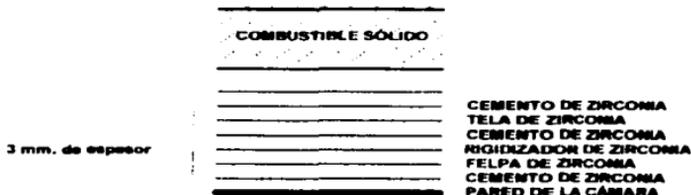
FIG. 1-4 DISEÑO DEL AISLANTE DEL COMBUSTIBLE SÓLIDO,
