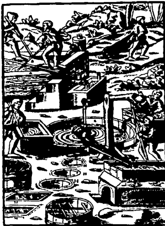
A-Tower B-Intoxicated ash C-Fluo D-Tower E-Reservoir F-Lamp G-Lead calson H-Wheel from axle into the water I-Vais in which tools are put
