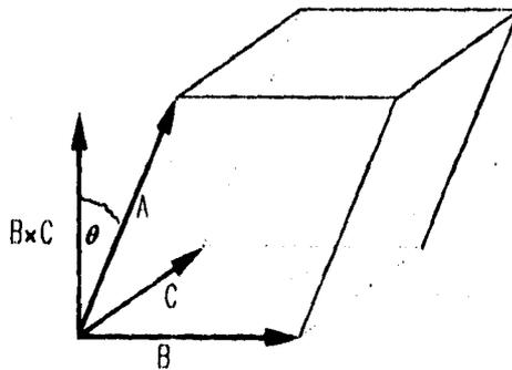
FIGURA 1.5L VOLUMEN DEL PARALELEPIPEDO  $|A \cdot (B \times C)|$
