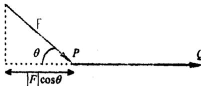
FIGURA 1.5JA TRABAJO REALIZADO POR  $F$  DURANTE UN DESPLAZAMIENTO  $\vec{PQ}$  ES
