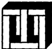
FIG. 2.3 TRANSFORMADOR TIPO ACORAZADO.
