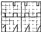
V_{CC} = 5V T_{HIGH} = 0.1 \mu s (PULSE) R_A = 10k\Omega C = 0.01\mu F For Time, Refer to the Model Time Tables in the General Timer Catalogue Tables 74 to 76
