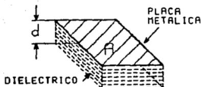
Fig.1-1 Capacitor elemental (6, fig. 8.6).
