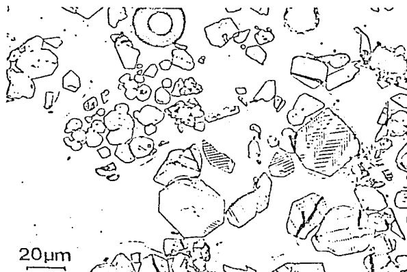
Fig. 4. Idem Fig. 3. Low leucite and small potash feldspar crystals in a glassy matrix. ROM.
