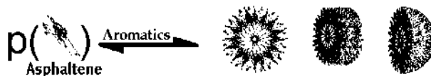
Fig. 4. Micellization (self-association) of asphaltene due to increase in aromaticity (polarity) of its medium.
