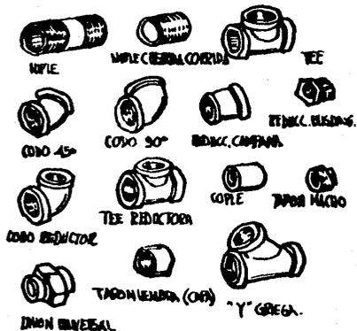
CONEXIONES CON LUERLO EN TUBOS
