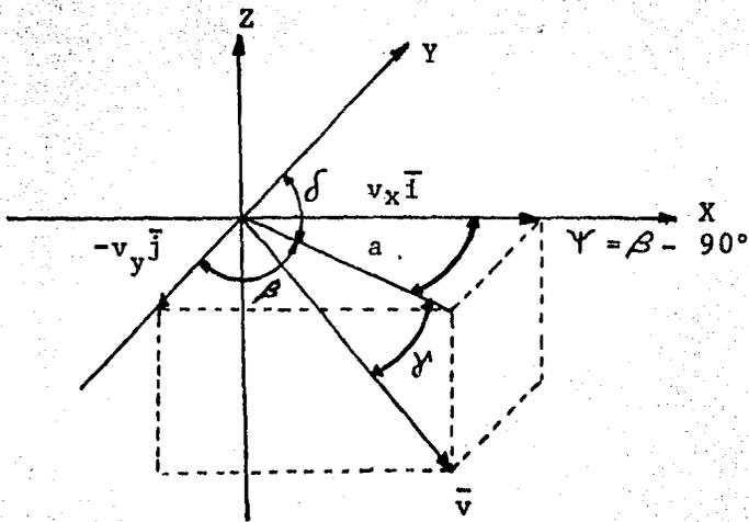
FIG. 2.4 Obtención de  $v_x$  y  $v_y$
