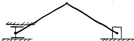
FIG.IV.1 MECANISMO BIELA-MANIVELA-PISTON
