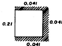
$$M (-) = C \times W \times \frac{B^2}{4} = 0.041 \times 1412.5 \times (4.00) = 926.6 \text{ kg/m}^2$$
